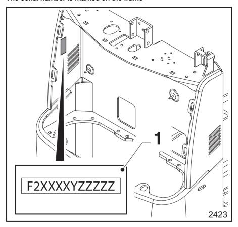
The truck's serial number is on the label (1) on the chassis frame.
