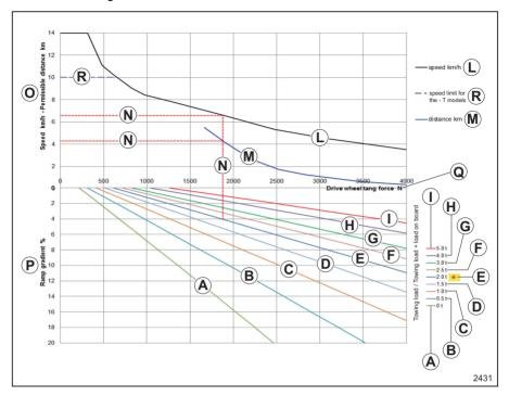
Towing load/Towing load + onboard load:
