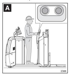
The image (A) shows the position of the operator on board the truck when using the back-rest fork controls.
