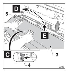
Push the toggle lever (4) inside the slot (C) to unlock the hood, then open the hood (3) as indicated (D).
