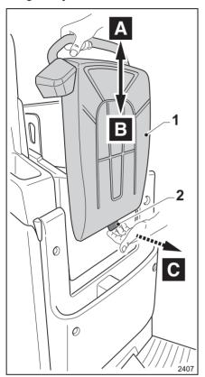
The height-adjustable seat backrest is optional and allows the operator to adjust the seat backrest according to their height to improve driving ergonomics.
