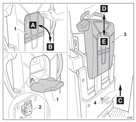
The foldaway seat is optional and allows the operator to drive while seated.
