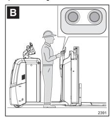
The image (B) shows the position of the operator when using the backrest fork controls from the ground.
