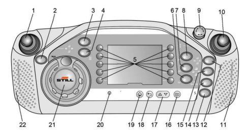
(1) Operating lever for hydraulics (in conjunction with the selection keys)
