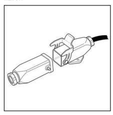
PIN 1 +12 V or +24 V PIN 2 + 0 V Max. 5 A
