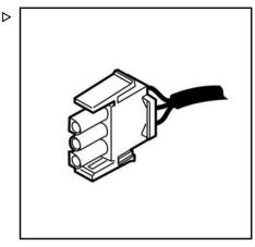
PIN 1 and PIN 2 +24 V PIN 3 + 0 V Max. 5 A
