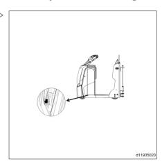
Push the moveable support to the side, and ▷ keep the moveable support close to the truck.
