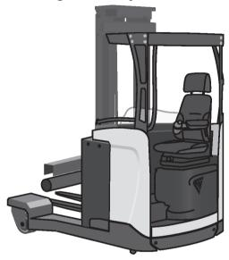
UFW Tergo (U\*\* Tergo) is an electric four-way truck, specially adapted for handling long and bulky loads and different types of load carriers. Driving in four directions is possible due to load wheel rotation. The truck operates both with the load carried in front of the straddle legs and with the mast retracted for minimum aisle width. The truck is used for stacking in different storage systems and for transporting load carriers.
