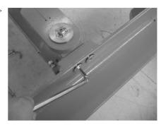
Tighten the clamping bolts of the rigid tiller using the dome nuts (tightening torque 30 Nm).
