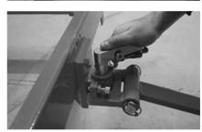
Evenly tighten the clamping bolts on the hinged tiller (tightening torque: 30 Nm) and secure the clamping bolts with nuts (tightening torque: 50 Nm).
