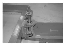
Insert the unmarked socket pin into the first frame in the drive direction. If necessary, drive in with a Teflon hammer.
