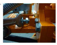
Secure the clamping bolts with nuts (tightening torque: 50 Nm).
