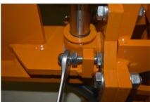
Secure the clamping bolts with nuts (tightening torque: 50 Nm).
