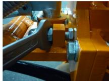
In order to the prevent the coupling (C) from turning, securely insert the rotation lock (A) on the hydraulic/pneumatic connection into the guard plate (B) (only with hydraulic and pneumatic systems).
