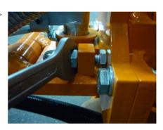
Release the coupling pin and remove the compensating hinge from the towing jaws.
