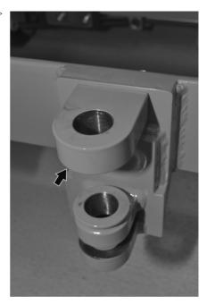
Insert the rigid tiller into the tabs on the second frame in the drive direction.
