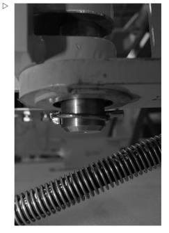
Tighten the screws for the tabs (two screws ▷ at both ends of the rigid tiller).
