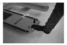
Push the trolley into the open side of the E frame until it reaches the stop. The E frame is raised by 40 mm and the trolley wheels turn freely. A prerequisite for this is sufficient pressure in the accumulator.
