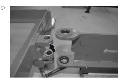
Do not tighten the screws. The tab must be loose.
