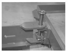
Insert the socket pin with the marking 5 (tab ▷ must be loose).
