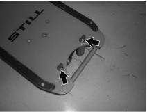
When the foot pedal is actuated (no interlock), the securing bolts must retract again.
