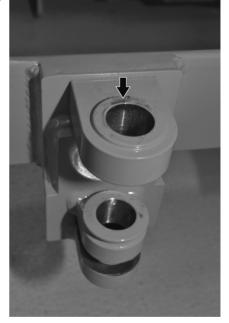
Insert the rigid tiller into the tabs on the first frame in the drive direction.
