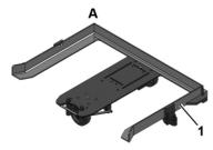
A Standard 1200 x 800 mm E frame with angular frame
