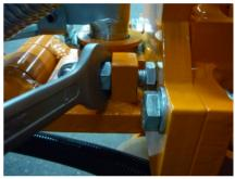
In order to the prevent the coupling (C) from ▷ turning, securely insert the rotation lock (A) on the hydraulic/pneumatic connection into the guard plate (B) (only with hydraulic and pneumatic systems).
