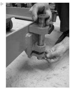
Screw on the tab (see arrow) for the second ▷ frame in the drive direction.
