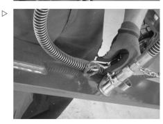
Connect the hydraulic hose line to the C frame.
