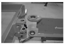
Do not tighten the screws. The tab must be loose.
