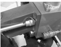
Fix the tiller support in a new position. To do this, tighten the mounting screws of the towing jaws by hand.
