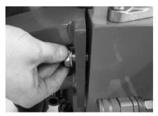
Tighten the mounting screws of the towing jaws (tightening torque: 200 Nm).
