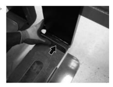
The securing bolt must extend at least 26 mm (locking position).
