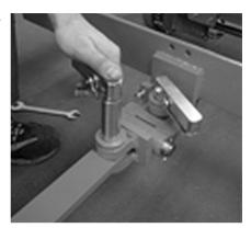
Loosen the nuts and the clamping bolts on the hinged tiller.
