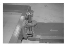
Insert the unmarked socket pin into the first frame in the drive direction. If necessary, drive in with a Teflon hammer.
