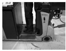
Enter the tow tractor and actuate the lifting/lowering switch on the tractor. All frames must lift or lower.
