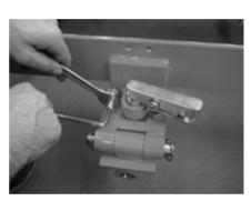
Release the coupling pin and remove the compensating hinge from the towing jaws.
