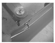
Tighten the clamping bolts on the rigid tiller (tightening torque: 30 Nm).
