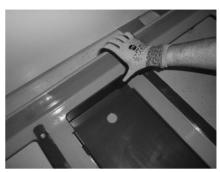
The securing bolts (see arrow) must extend pat least 26 mm (locking position).
