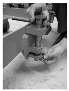
Screw on the tab (see arrow) for the second prame in the drive direction.
