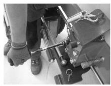
Insert the tiller into the support mounting and push in the bolt. Secure the bolt using the linch pin.
