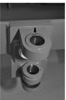
Insert the rigid tiller into the tabs on the first prame in the drive direction.
