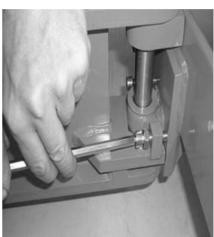
Secure the clamping bolts with nuts (tightening torque: 50 Nm).
