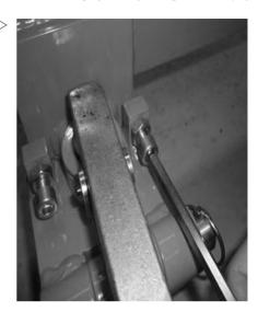
Tighten the nuts on the clamping bolts (tightening torque: 50 Nm).
