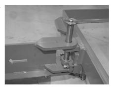
Insert the socket pin with the marking 5 (tab pmust be loose).
